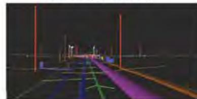
The BIM models of the networks are federated at the end of the modelling phase: based on the federated BIM model, QA & QC procedures are performed to check the model's consistency to the survey data and the client's requests
